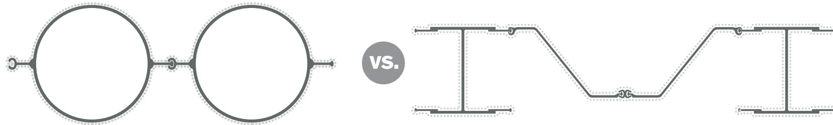
Furthermore, the interior of the pipe can be sealed off (capped or filled) from oxygen infiltration to avoid corrosion on the inside surface. Also, concrete can be poured inside the O-Pile itself, thus further increasing strength while preventing oxidation or corrosion on the interior surface. This contrasts with a combined sheet pile system, which has all of its surface faces exposed to corrosive elements.
