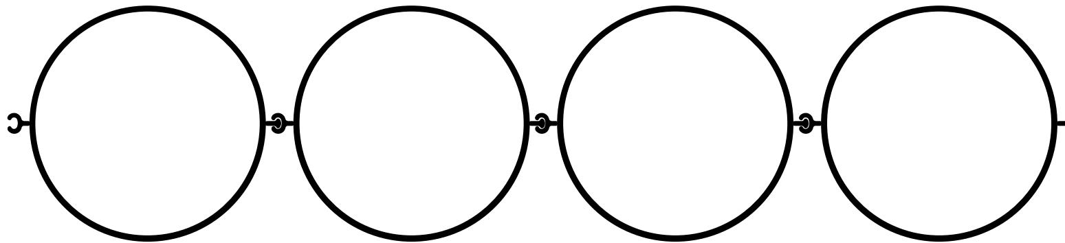
O-Pile is a dynamic, cost-effective, contiguous pipe-to-pipe system that allows you to drive predictably into pure rock, if necessary, as well as dial in your corrosion and bending moment needs separately. O-Pile is versatile and readily available, as you can use your local pipe plant or supply—no need to bring the majority of the steel from Luxembourg anymore.
