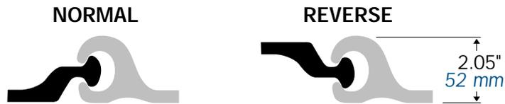
The reversed interlock arrangement can be utilized to bypass obstructions when they are encountered along the driving line or to shift the driving line.
