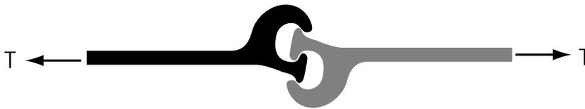
Tensile Diagram For Properly Interlocked PS Sections
