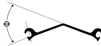
Small cells constructed with bent web piles must have half of the piles bent with the fingers inside and half with the fingers outside.
