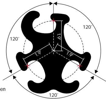
Wye Connector for Open Cell construction.
