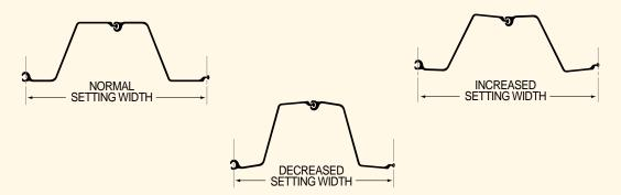
Sheet piling supplied with the interlocks crimped or welded does not offer this advantage.
