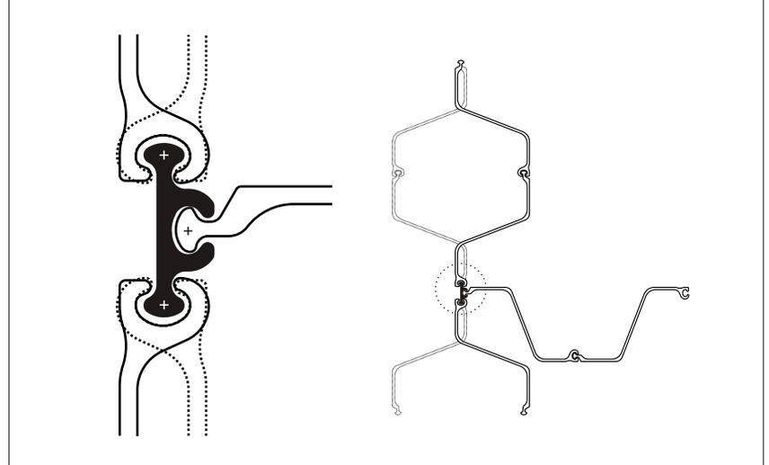
**Improper Interlocking Combinations**
