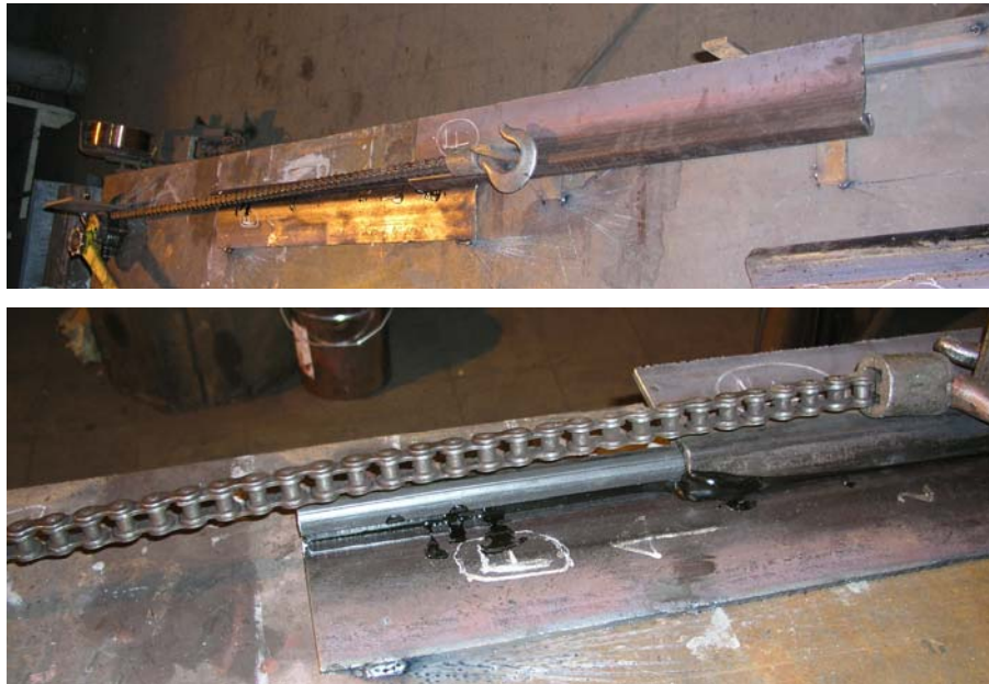
Figure 8: Insertion of the panels (LARSEN Interlock)
