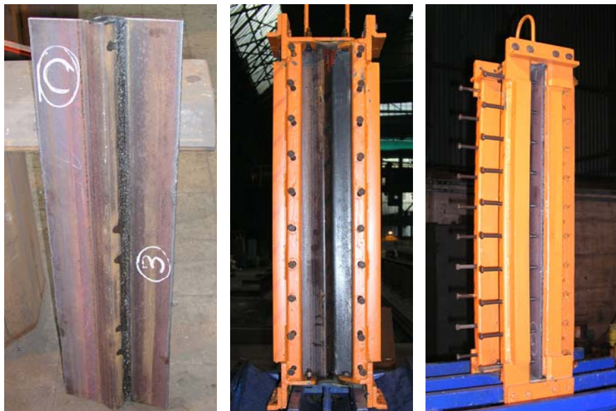
Figure 2: Test Setup with specimen a) Specimen b) Front view c) Side view
