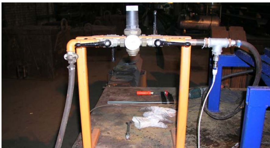
Figure 3: Pressure control system with manometer
