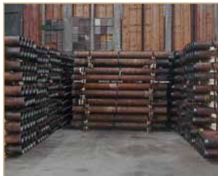
Female and male casing cut and bundled to specifications
