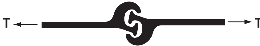
Tensile Diagram For Properly Interlocked PS Sections
